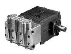
T Series 76, Triplex Plunger Pump, Solid Shaft – Forged brass manifold with an exclusive lifetime warranty. The industry's choice for high flow applications, over sized connecting rods for maximum life. Max. Inlet Pressure: 125 PSI Max. Fluid Temperature: 165° F Inlet Port Thread: 1" NPT-F Discharge Port Thread: 1/2" NPT-F Shaft Diameter: 1.378 in./35 mm Pump Dimensions: 15.6" x 14.0" x 9.5" Max. Inlet Vacuum: 7 ft. water (6.2 in. Hg) Crankcase Oil Capacity: 91.0 oz.
